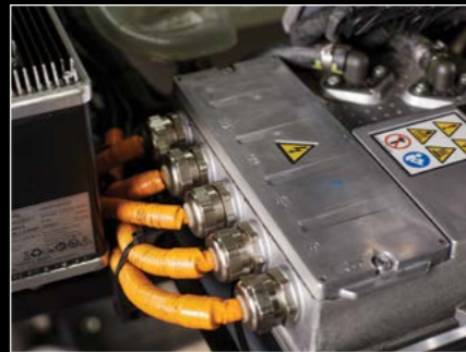
When getting on and off the kart, it is better to avoid stepping on the orange high voltage cables (350 Volt) which are connected to the control unit and are in any case in a fairly protected position
