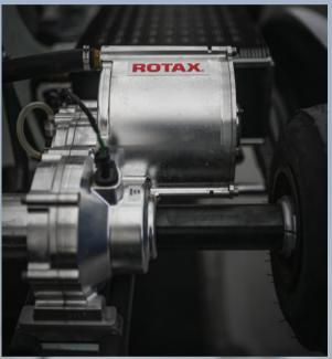
The orange electric cables are the ones where the high voltage current passes: it is therefore better to respect them, when you get in and out of the kart or you are working on it... The electric motor developed by **Rotax integrates** the transmission as already happens for the DD2 engines, so much so that it requires the use of the same type of frame, produced by Sodikart
