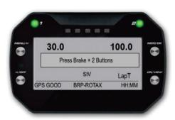
The instrument specially developed for the Rotax Project E20 can signal isolation problems of the electrical apparatus even with red lights. It also shows the charge and temperature status of the battery pack, as well as the gear between N, R and D (respectively neutral, reverse and drive) which is activated via the buttons on the steering wheel
